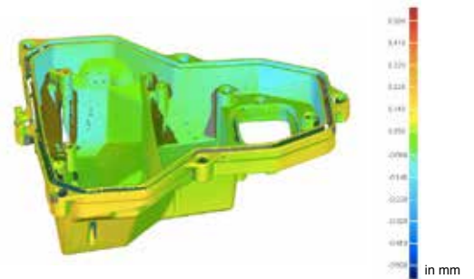
DC charger housing shows minimal dimensional change after automotive thermal/humidity cycling, with 95% of points within ±150µm of initial
